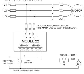
Set the VOLTAGE adjustment to the nominal operating voltage. Models 22 and 22M will auto-range to either the 190-240VAC or 380-480VAC scale. Set the UNBALANCE, RESTART, and TRIP adjustments as required for the application.
