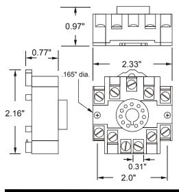
The Model 51X016 11-Pin Socket is a surface or DIN-rail mount socket.
