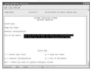
To clear Alarm Logs, press the "l" key and then hit Enter.
