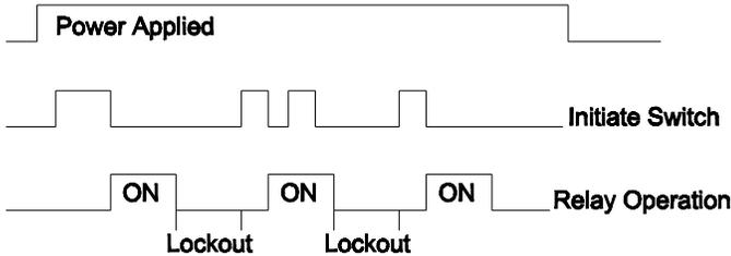
Power is applied to the coil all the time (Pins 2 & 7). When the initiate switch is closed, nothing happens. When the initiate switch is opened, immediately the relay will energize for the Interval time period. At the end of the Interval "ON" time, the relay will de-energize and remain de-energized until the total time period (Lockout) has elapsed.
